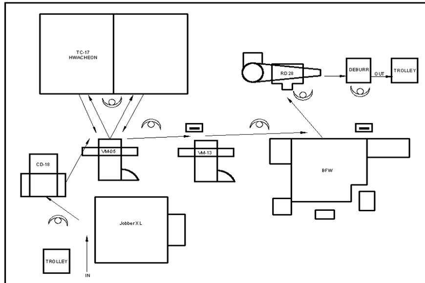
**Figure 3, Machining cell layout (After)****STANDARDIZATION OF WORK**
